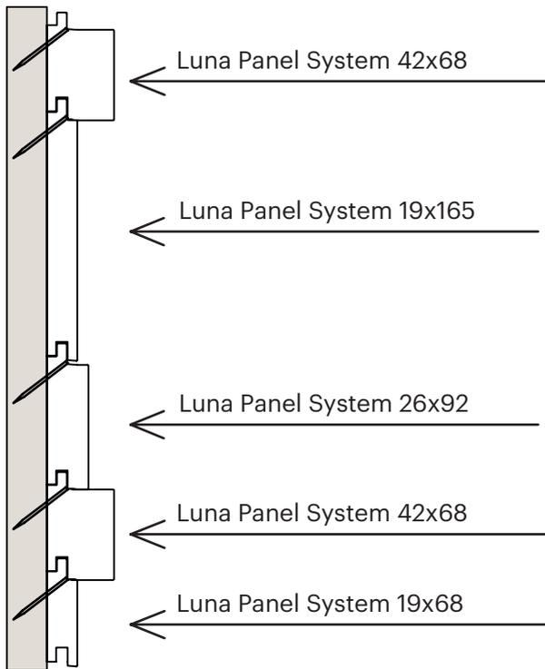
Stainless steel nail or screw length 40-45 mm.
